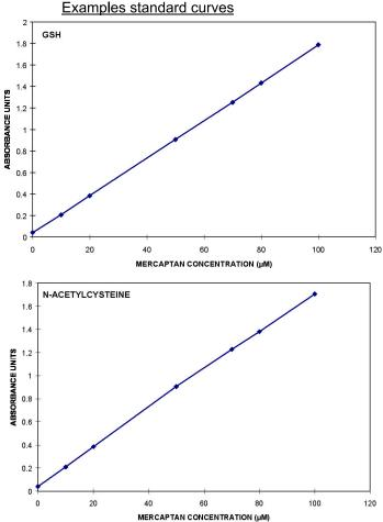
Figure 2: Example of standard curves obtained at 356 nm at 25°C.
