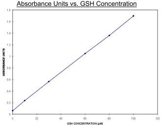
Figure 1: Example of standard curve obtained at 400 nm at 25°C.
